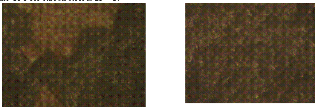
Figure 2: Surface analysis of carbon steel after 3 days of immersion in solution containing \text{FeCl}_3 at 25°C.
